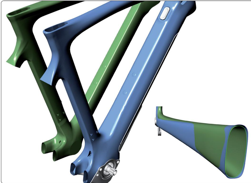
In these pictures is visible a comparison between the new Nytro frame (light blue) and a traditional road bike (green). Dimension of the down tube and bottom bracket are visible wider in order to provide the right frame rigidity values and integrate the Fazua Evation System.
